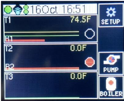
**Large circle** - Indicates the connection between the Mainboard and the LCD screen. Should be green and may indicate an issue if it stays red.
